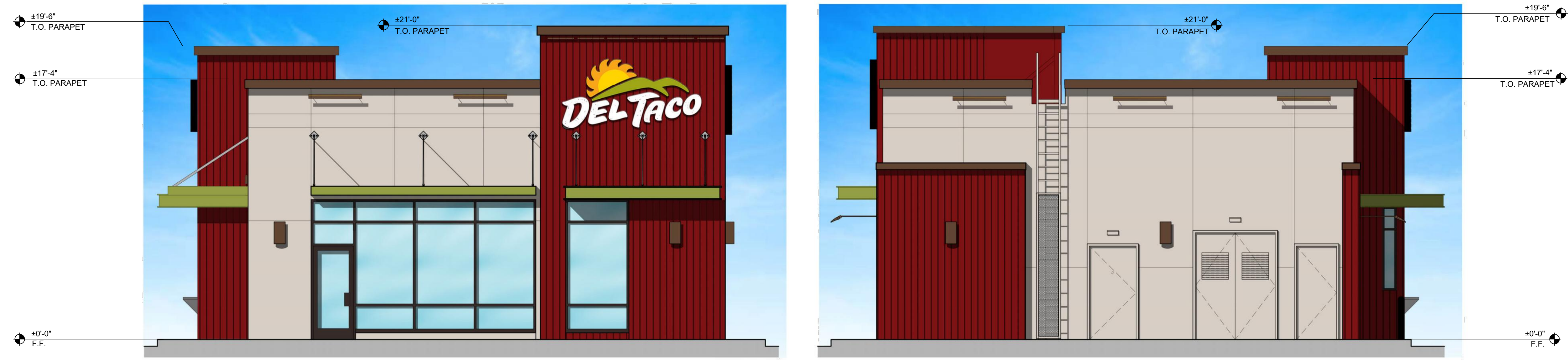
4 NORTH ELEVATION 1/4" = 1'-0" 3 SOUTH ELEVATION 1/4" = 1'-0"
